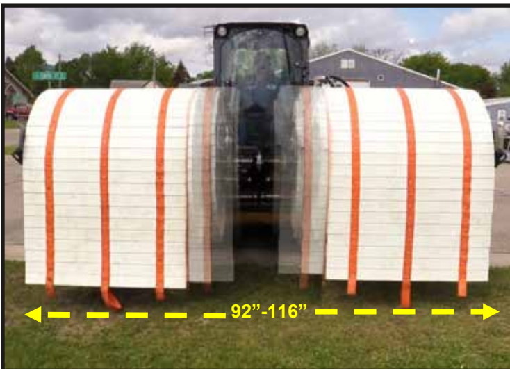
Single Spool Attachment Designed for smaller loader carries 48" wide Trax
