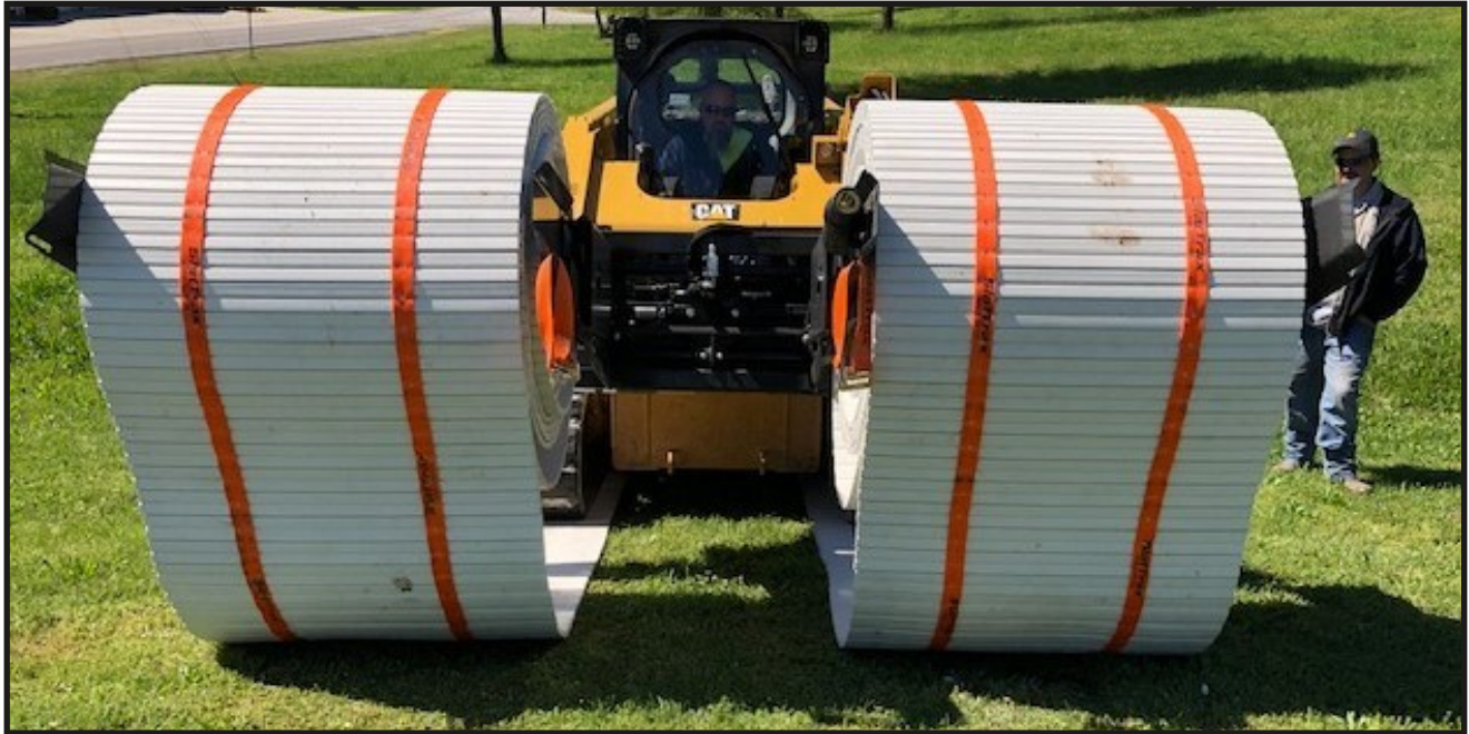
Dual Spool Attachment for skid loaders with standard plate mount and hydraulic operation Capacity of 100 to 125 LF of dual Trax comprised of 12.5' linked sections
